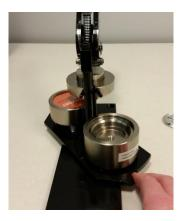
e. The empty die now in front of you is called the crimp die. Place a pin back in the crimp die with the sharp edge facing <u>up</u>. You should be seeing the zigzag side of the pin back.
