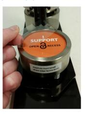
d. Once your shell, paper design, and mylar are in place, spin the pickup die underneath the punch.
